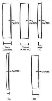
Positions for Measuring Camber of Shapes
